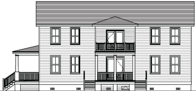
WEST (DRIVEWAY SIDE) ELEVATION 1/4" = 1'-0"
